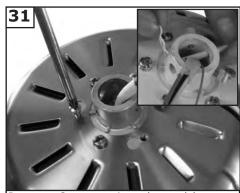
Remove 2 screws in yoke and keeper then cross pin (see insert). Remove 3 screws with keyhole slots from top of fan.
